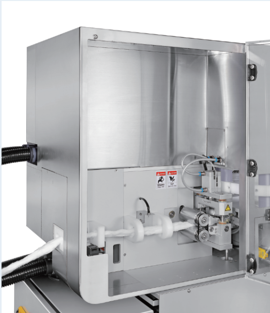
Cotton pre-feed device features smooth and nonstop cotton feeding.
